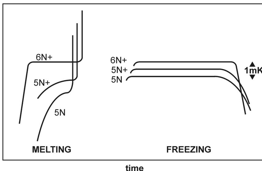
For all but Primary Laboratories, it is quicker, simpler and easier to use fixed point cells during their melt. Slim Cells are all 6N<sup>+</sup> pure so that the melt curve is very flat.
